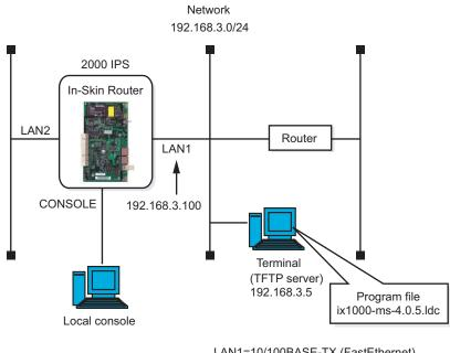
LAN1=10/100BASE-TX (FastEthernet) LAN2=10BASE-T (Ethernet)
